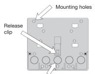
Conduit knockouts on back and bottom
