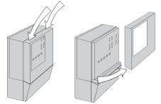
2. Loosen screws at front and pull wiring cover straight out.
