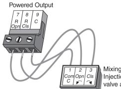
Mixing or Injection valve actuator
