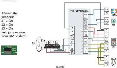
The WiFi Thermostat 563 operates a first stage radiant floor and a second stage fan coil for heating, and two-stage air conditioner for cooling and dehumidification, and a humidifier.
