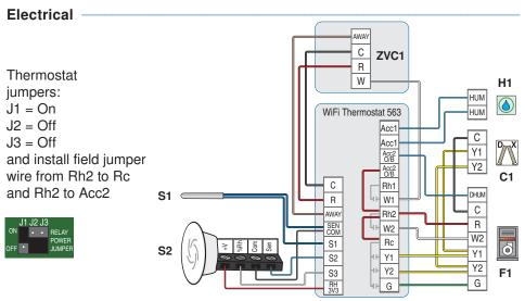
The WiFi Thermostat 563 operates a first stage radiant floor and a two-stage air-to-air heat pump for heating, cooling, and dehumidification, a backup electric heater, and a humidifier.
