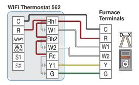
The WiFi Thermostat 562 operates a first stage radiant floor and a second stage furnace for heating, and an air conditioner for cooling.
