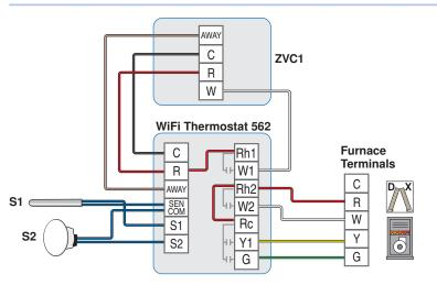
The WiFi Thermostat 562 operates a first stage radiant floor and a second stage fan coil for heating, and an air conditioner for cooling.
