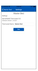
• Click the button to view the thermostat model, tekmarNet address and change the thermostat name.
