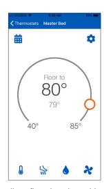
• Click the floor heat  $\frac{1}{m}$  button to adjust the floor heating temperature (only available for radiant floor heating with a floor sensor).
