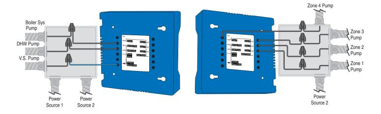
**Rear Line Voltage Wiring Diagram**
