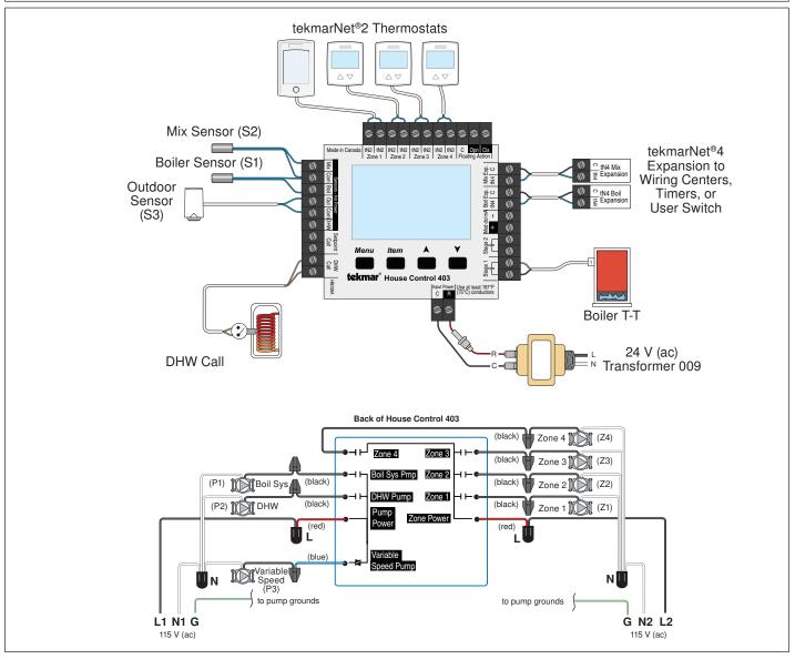
**Description:** The House Control 403 operates a modulating boiler with indirect Domestic Hot Water. Mixing is performed with a three-way floating action mixing valve, which supplies a reset water temperature to four mix temperature hydronic zones. Four boiler water temperature zones shown are operated by a Wiring Center through the tN4 Boil Expansion terminals.
