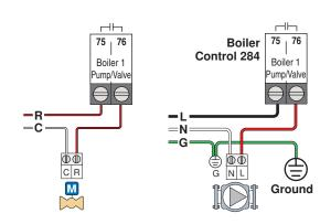
An indirect DHW pump requiring up to 230 V (ac) 5 A, 1/3 hp can be switched through the IDHW Pump terminals.
