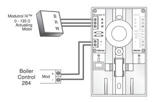
V9055™ 0 - 135 Ω Actuating Motor (O) Boiler Control 284
