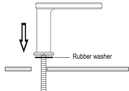
**2** - Slip the spout mounting hardware back onto the spout. First the notched rubber washer, then the notched metal washer and lastly the brass lock nut. Hand tighten the lock nut.
