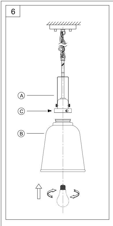
6. Attach glass (B) to fixture (A) using thumb screw (C) to secure tightly.
