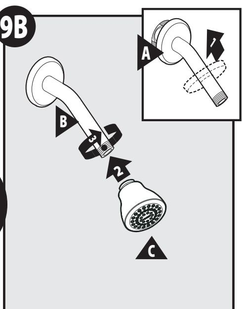
**Plastic Shower Ball:** Slide Shower Arm Escutcheon (**A**) over Shower Arm (**B**). Remove any debris from the Shower Arm to ensure proper flow. Then, simply thread Shower Head (**C**) onto Shower Arm (**B**).
