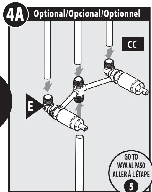
If soldering copper tubing (CC) into valve (E) insert  $\frac{1}{2}$ " copper tubing into the hot and cold water inlets and the shower riser and tub drop outlets.
