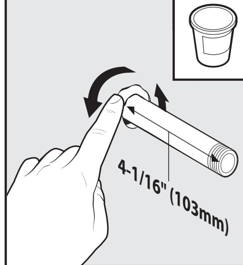
The threaded pipe for the tub spout should protrude 4-1/16" out from the finished wall. Apply a sealant between the wall opening and the pipe.
