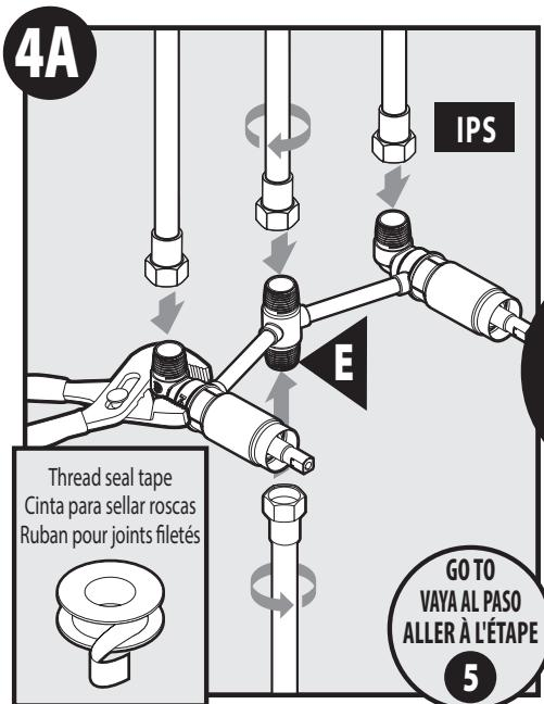
This valve (E) can be plumbed using threaded connections (IPS). The water inlets, the outlets to the tub spout and to the showerhead are  $\frac{1}{2}$ " male pipe thread. Use thread seal tape when making these connections. Wrap the tape onto the threads in the same direction the adapter will thread on. Use adjustable pliers or a pipe wrench to hold the valve body when tightening the connections.
