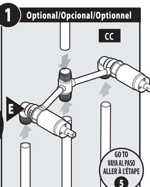
If soldering copper tubing (CC) into valve (E) insert 1/2" copper tubing into the hot and cold water inlets and the shower riser and tub drop outlets. Then, go to **Step 5**.
