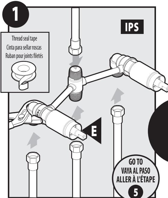
This valve (E) can be plumbed using threaded connections (IPS). The water inlets, the outlets to the tub spout and to the showerhead are 1/2" male pipe thread. Use thread seal tape when making these connections. Wrap the tape onto the threads in the same direction the adapter will thread on. Use adjustable pliers or a pipe wrench to hold the valve body when tightening the connections. Go to Step 5.
