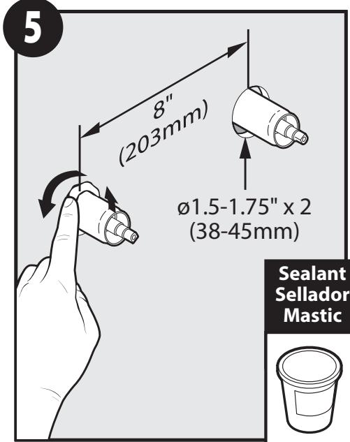
Apply plumbers putty or other sealant to the area surrounding the wall tubes.
