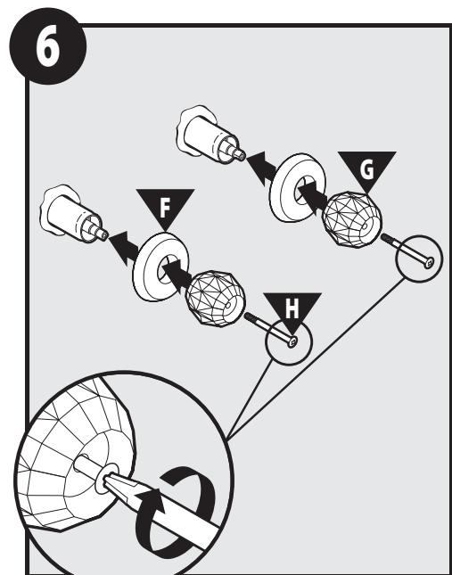
Slide wall tube escutcheons (F) over wall tubes. The cold handle (G) has a "C" stamped inside as shown and is to be installed on the right side. The hot handle (H) has a "H" stamped inside and is to be installed on the left side. Thread screws (J) into handles.
