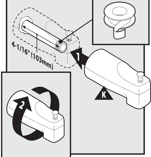
Wrap thread seal tape counter clockwise on the pipe threads. Thread the tub spout (K) onto the pipe.
