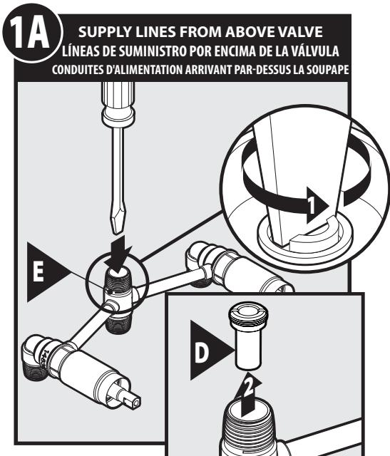
Position the valve as seen in Step 1B. Locate and remove the Flow Director (D) in the top outlet of the valve using a flat head screwdriver.
