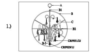
Step.2: Hang the crystal (CRP031/2J /CRP029/1J) on the metal cup(B2)
