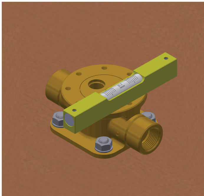
Ensure valve is perfectly level
