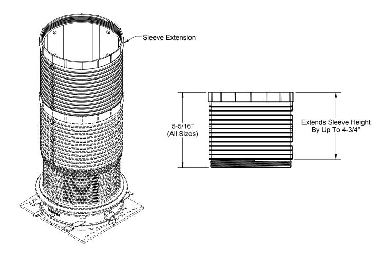
The HOLDRITE® Hydroflame Pro Series "Sleeve Extensions" (#HFPE1 - #HFPE6) are available to fit a wide variety of Sleeve combinations, from 1" thru 6" sizes. Each extension adds up to 4-3/4" of height in 1/4" increments. No coupling is needed! Height markings are shown on each part, in both U.S. and metric.
