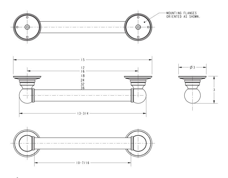
MEETS OR EXCEEDS ASTM F446 STANDARDS AND CONFORMS TO ADA GUIDELINES.
