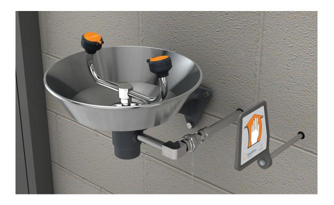
**Application:** Freeze-resistant eyewash for wall mounting. Valve and supply line are located behind wall in heated area to prevent freezing. Self-draining valve permits water to drain completely from unit after use. Since unit is intended for use in cold weather conditions, consideration should be given to supplying unit with tempered water in accordance with ANSI Z358.1-2014. See "Tempering Valves" section for more information.
