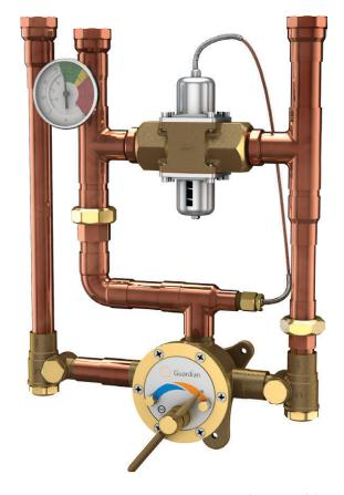
**IMPORTANT:** Pursuant to ANSI Z358.1-2014, the water delivered by emergency equipment should be "tepid". Tepid is defined as moderately warm or lukewarm, and is generally considered to be between 60°F (15°C) and 90°F (32°C). However, in certain circumstances, a chemical reaction may be accelerated or otherwise affected by the water temperature. Please consult with a medical advisor to determine the optimum delivered water temperature prior to specifying, installing or using a tempering valve.
