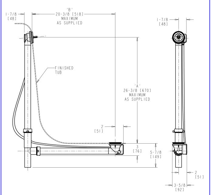
DIMENSIONS ARE IN INCHES AND [MILLIMETERS].
