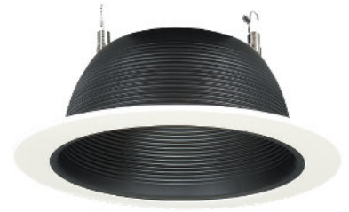
1126-15 RECESSED TRIM Black Steel Baffle White Steel Trim Maximum Wattage: 75w PAR30L 65w BR30 50w PAR30S 13.5w A19 15w PAR30L 15w BR30
