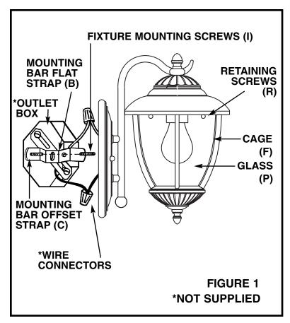
WARNING: TO REDUCE THE RISK OF FIRE, ELECTRIC SHOCK OR PERSONAL INJURY, MOUNT TO OUTLET BOX OR SUPPORTING SYSTEM ABLE TO SUPPORT THE WEIGHT OF THE FIXTURE.
