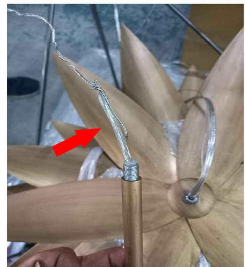
9. SLIP WIRE OVER THE STEM
