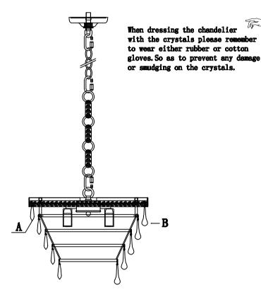
1. Hang the crystal (A) and the crystal (B) on the first circle to the fifth circle of the Lamp Frame as shown in the figure.
