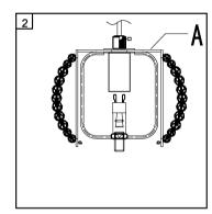
3.Screw part glass(B) onto the lampbody(A) secure with screw.
