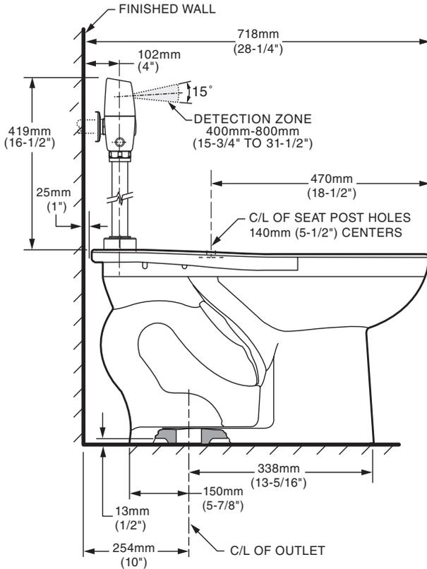
\*Note: The Critical Line (-C-L-) on Vacuum Breaker must typically be a minimum of 6" (152mm) above fixture. Consult Codes for details.
