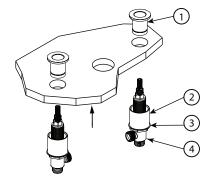
Remove top fastening nut and washer (1) from the lavatory valve. (NOTE A: All lever handle sets are supplied with one righthand valve and one left-hand valve. Install valve with blue dot o the cold side [Round handle sets are supplied with two hot valves that turn in the same direction]). Insert valve from below through hole in lavatory or countertop.
