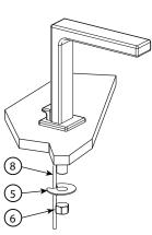
Insert spout base nipple into center hole in lavatory or counter top. Install stainless washer (5) nut (6) on spout nipple and tighten. Place pop-up knob rod (8) through spout.
