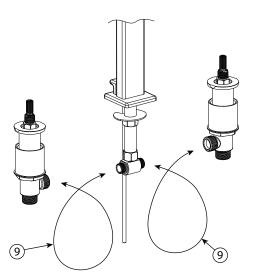
Connect stainless steel flex lines (9) from valve outlets to spout tee (7). Flex lines should be looped as shown in diagram. FLEX LINES MUST NOT BE KINKED. Adjust valves and or spout teeto eliminate any kinking in the flex lines. Install escutcheons onto the valves and hand tighten. DO NOT OVER-TIGHTEN. Install handles onto valve stems.
