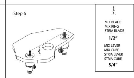
Set valve to proper rough-in height "A", by adjusting bottom - fastening nut. Secure valve by tightening top fastening nut. Repeat procedure for the second lavatory valve.
