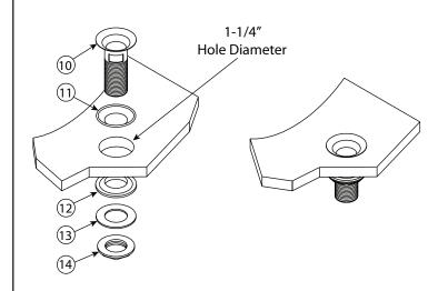
Insert drain rim (10) into the basin placing the Teflon washer (11) under the rim. From below slip on washer (12) onto the bottom thread of the drain rim and secure to basin with drain nut and washer (13 and 14).
