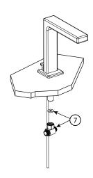
Install spout tee assembly (7) as shown in diagram.
