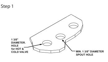
Should a counter top need to be drilled, please reference the diagram above.
